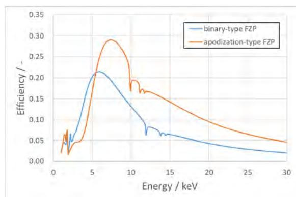
Fig. 2. Diffraction efficiency of FZPs.
