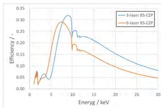
Fig. 1. Diffraction efficiency of BS-CZPs.
