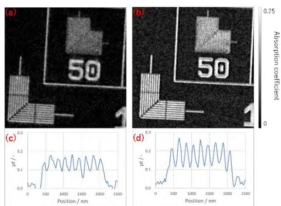
Fig. 3. X-ray chart patterns: (a), (c) conventional optics (exposure time: 150 ms), (b), (d) new optics (exposure time: 20 ms). (a) and (b) are  $\mu\text{t}$  images, (c) and (d) are line profiles of 100 nm L&S.
